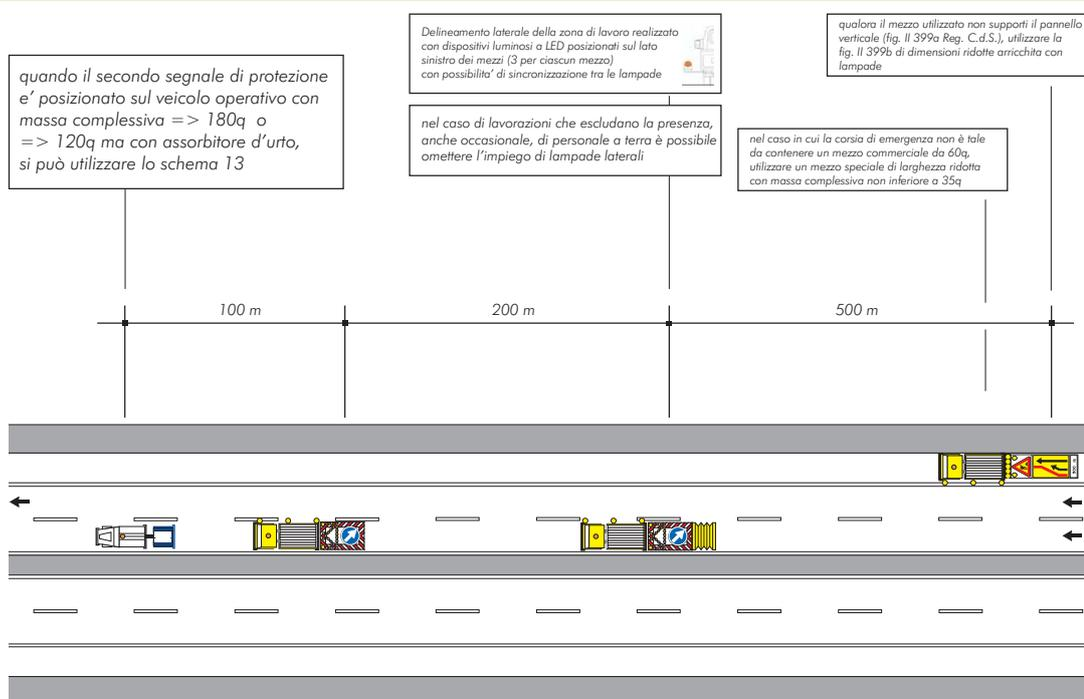
**SEGNALETICA MOBILE A PROTEZIONE DI VEICOLI SPECIALI IMPIEGATI PER LAVORI, CONTROLLI, SONDAGGI E VERIFICHE DI RAPIDA ESECUZIONE, CHIUSURA DELLA CORSIA DI SORPASSO**
