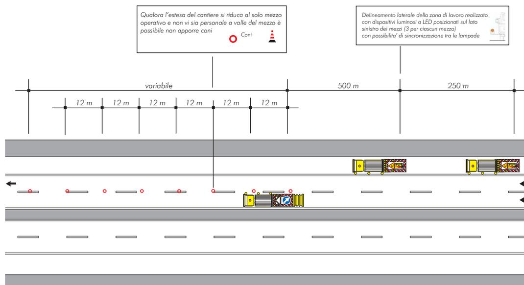
**CANTIERE IN LENTO AVANZAMENTO, CHIUSURA DELLA CORSIA DI SORPASSO CON PRESENZA ESTEMPORANEA DI PERSONALE A TERRA**
